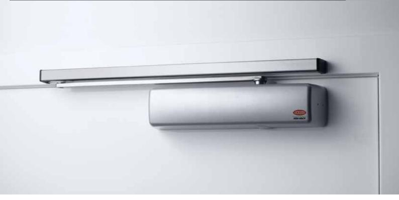
The Lockwood 2516EMC is a small single door electromechanical hold open device system with a sliding arm. It is applicable for places, where fire doors are constantly kept open. The door is kept open at a selected angle. If fire breaks out, the door is closed, preventing smoke and flames from spreading. Applications for 2516EMC include hotels, office buildings and other fire doors where hold open function is needed.
