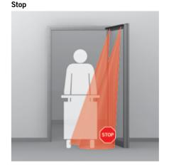
Infrared safety sensors are active infrared sensors and designed to detect all static and moving obstructions, either people or objects, within their detection range.
