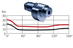
Force curves, spring strength EN 3 Opening torque
