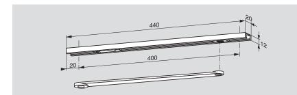
The DORMA G 96 N20 slide channel pack includes the arm, slide channel, slide block, cushioned limit stay and fixing screws, and can be combined with both door closer sizes in the DORMA ITS 96 range. The DORMA G 96 N20 slide channel is adjustable to K8/K12.
