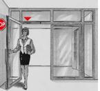
Cushioned limit stay simply slides into the slide channel. Adjustable between 80° and max. 120°. Also suitable for retrofitting.
